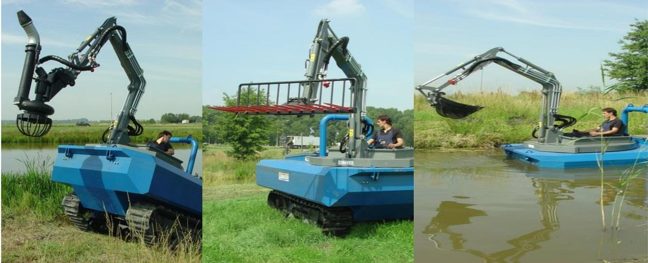
The C550 has a balanced undercarriage where power, grip and limited ground pressure are combined. Because the turret with hydraulic arm is also fitted to the same chassis, no mechanical forces are superimposed onto the hull, whilst keeping it as light as possible. Because of the 200 degrees revolving operators compartment, the driver always has the work in plain sight and acts as counterweight as well.
