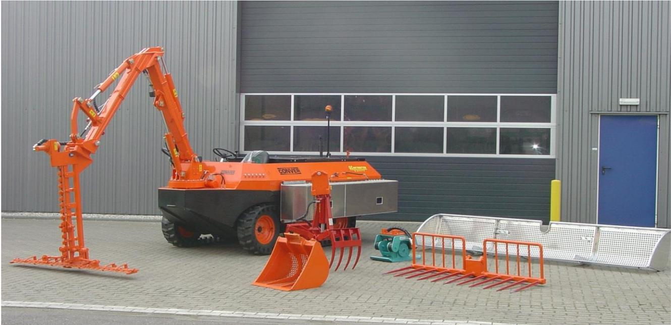
This multi-functional do-it-all for on land and in water is executed with hydraulic connections for application of various hydraulic and mechanical attachments.
