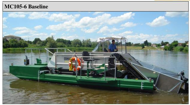
Medium size main hull and separate side pontoons for easy road transport. No fixed cabin for easy passage under low bridges. High capacity due to fast self-unloading system.
