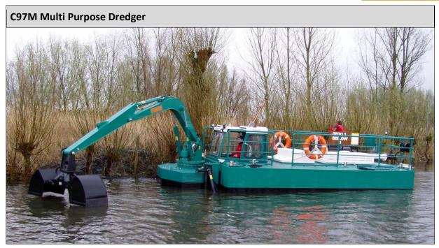
The Conver C97 Multipro is a versatile Multi Purpose Dredger that has been developed to provide the user with a versatile tool that combines productivity and efficiency with portability and the ability to operate and move in water and on land.
