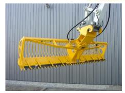
**DP200-8"hc** with hydraulic cutter head, 600mm cutter
