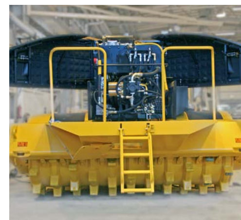
Simplicity in design provides a high uptime for TANA compactors. Easy access to the power pack from the rear saves time on routine maintenance operations and checkups. The optional ladders add usability for daily use.
