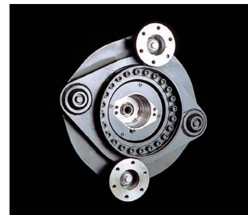
The swing frame construction (pat.) by TANA protects the final drive gearbox, thus increasing reliability and maximizing uptime of the machine.
