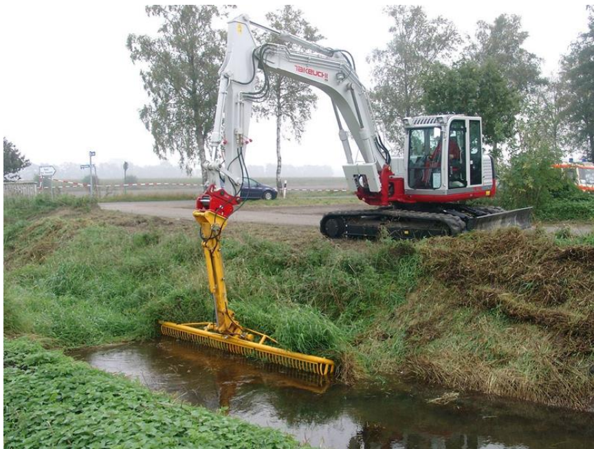
Midi-excavator with arm-extension. Extension not required for the lengthened Amphitrax arms.
