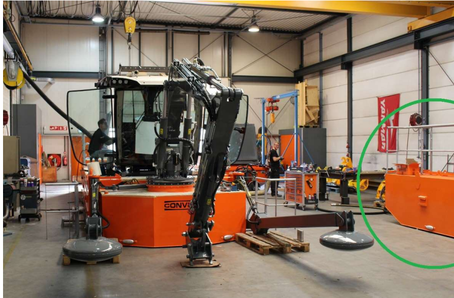
Encircled part is the detachable floater near the hull for easy transport
