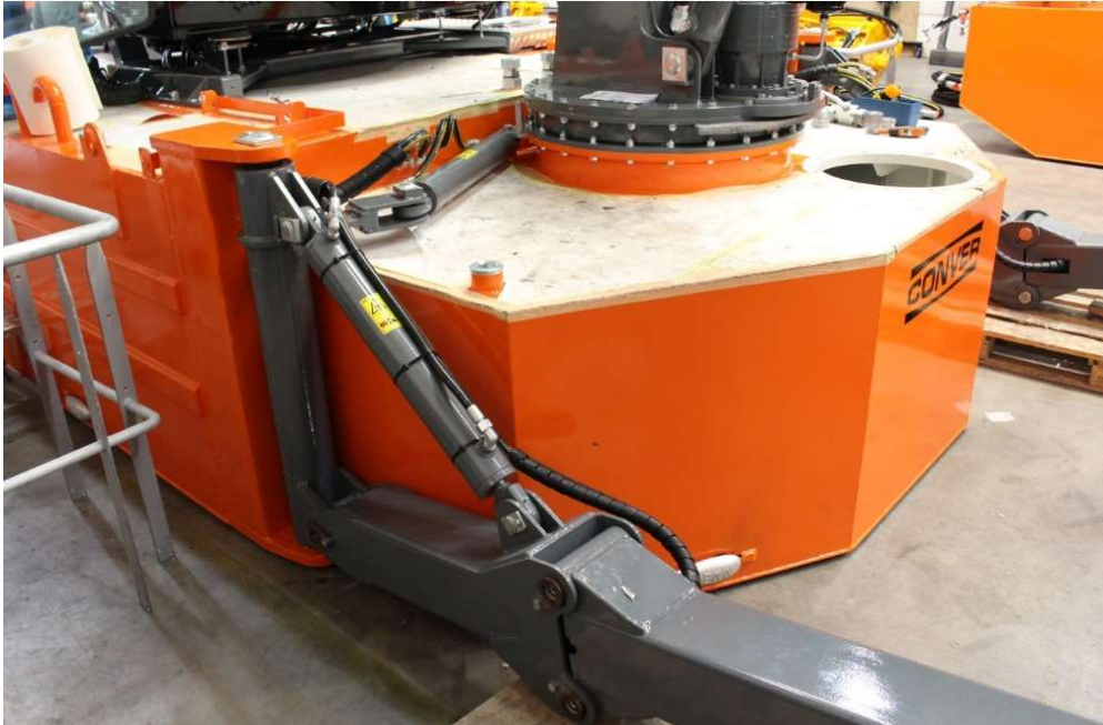
Easy to take off the stabilizer (Stabilizer Mechanism)
